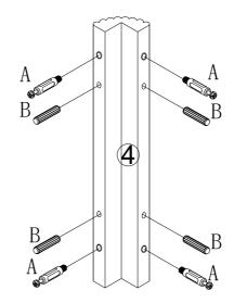
No. A Quantity:16 Pcs Cam Lock Dowel 8\*28mm No. B Quantity:16 Pcs Dowel 8\*30mm
