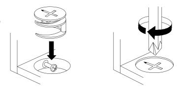
Turn cam lock clockwise to tighten.
