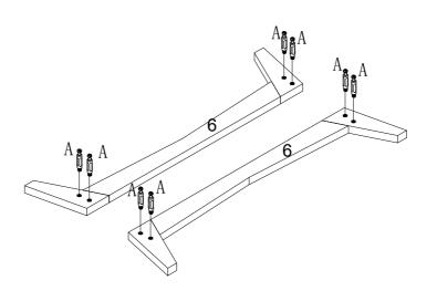
No. A Quantity: 8 Pcs Cam Lock Dowel 8\*28 mm
