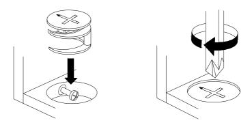
Turn cam lock clockwise to tighten.
