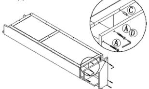
Step 3: Fix  ${\mathfrak T}$  and  ${\mathfrak B}$  bottom side panels with "A"screws and use "B"screws to connect  ${\mathfrak G}$  bottom panel
