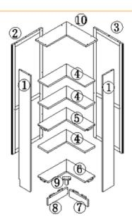
Step 3: Use Cdisk dowels and fix with "A"screws to install the top panel
