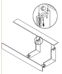
Step 2: ②back panel rests on ③back panel and is fixed with "A"screws, and at the same time,
