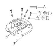
将底盘放置在座垫的中心位,使用五金D. E对准座垫的孔位锁紧固定 Place the chassis at the center of the seat cushion, and use hardware D.E to align with the hole of the seat cushion to lock and fix
