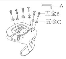
将椅背放置在座垫的承台位,使用五金B. C通过椅背对准座垫的孔位锁紧固定 The seat back is placed on the cushion cap position of the seat cushion, and the hardware B.C is used to align the seat back with the hole position lock of the seat cushion.
