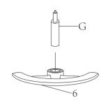
将气压棒装入脚踏的中心孔 The gaslift must be placed from top 再将气压棒装入椅脚的中心孔 to bottom into the footrest as the
