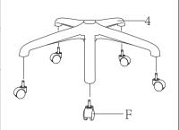
把椅轮分别装入椅脚的五个脚孔。 Fit the castors into each of the five holes of base.
