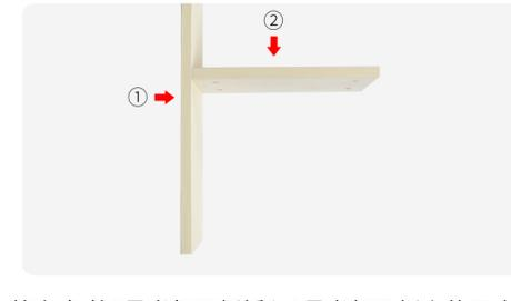
第六步 将2号书架面板插入1号书架面板上的三合一螺杆D上, 将偏心轮E固定, 先不要拧紧 6. Insert the No.2 bookshelf face ply into the screw D on the No.1 ply, then fix the part E, don't tighten it too tight.
