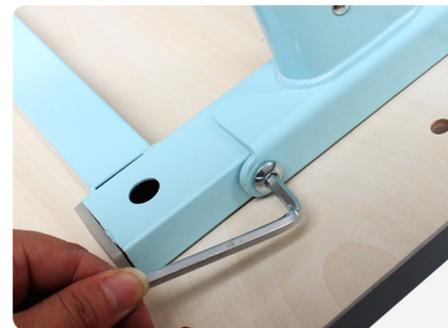
第一步 用螺丝A将一边的桌腿固定到桌面上(螺丝先不要拧紧) 1. Fix the leg (one by one) on the table with screw A, and don't tighten it too tight.
