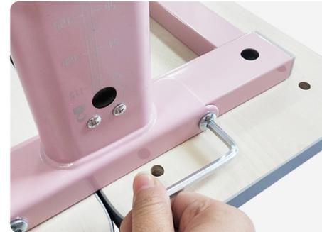
第一步 用螺丝A将一边的桌腿固定到桌面上(螺丝先不要拧紧) 1. Fix the leg (one by one) on the table with screws A, and don't tighten it too tight.
