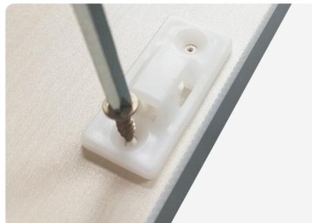
第十五步 此位置安装防倒器的,若需安装防倒器,防倒器说明书见防倒装置配件包 15.If you want to install the anti-reverse parts, pls refer the relevant directions .
