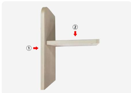
第七步 将2号书架面板插入1号书架面板上的三合一螺杆D上,将偏心轮E固定,先不要拧紧 7.Insert the ② into the ① (pass through D), then fix the part E, don't tighten it too tight.
