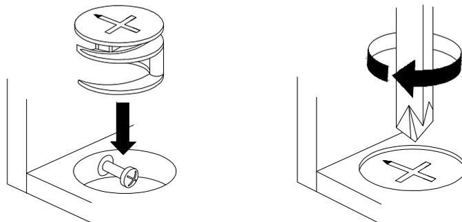
Turn cam lock clockwise to tighten.
