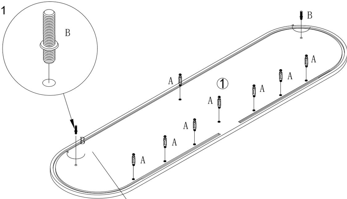
Please note the screw B have different thread length at both side, ensure the shorter thread side towards down as drawing shows.
