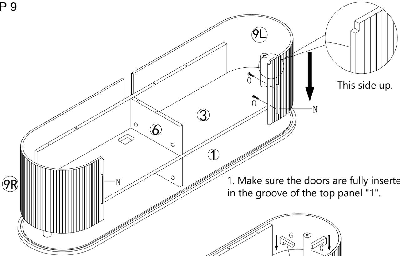
1. Make sure the doors are fully inserted in the groove of the top panel "1".
