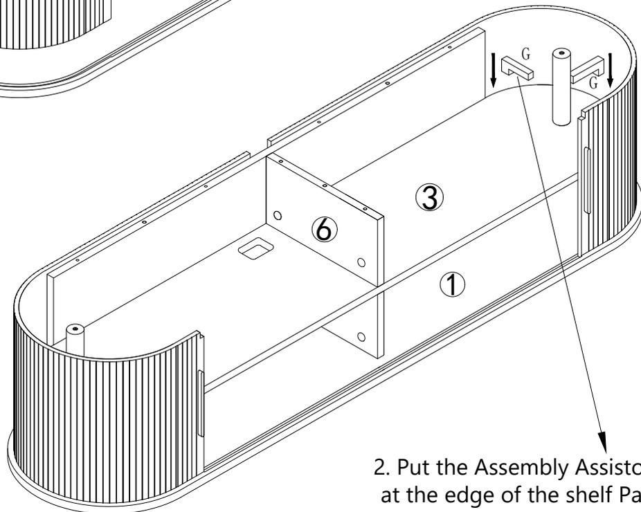
2. Put the Assembly Assistor "part G" at the edge of the shelf Panel "3"
