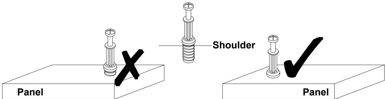
Tighten quickfit until shoulder is flush with panel. Do not overtighten or undertighten.
