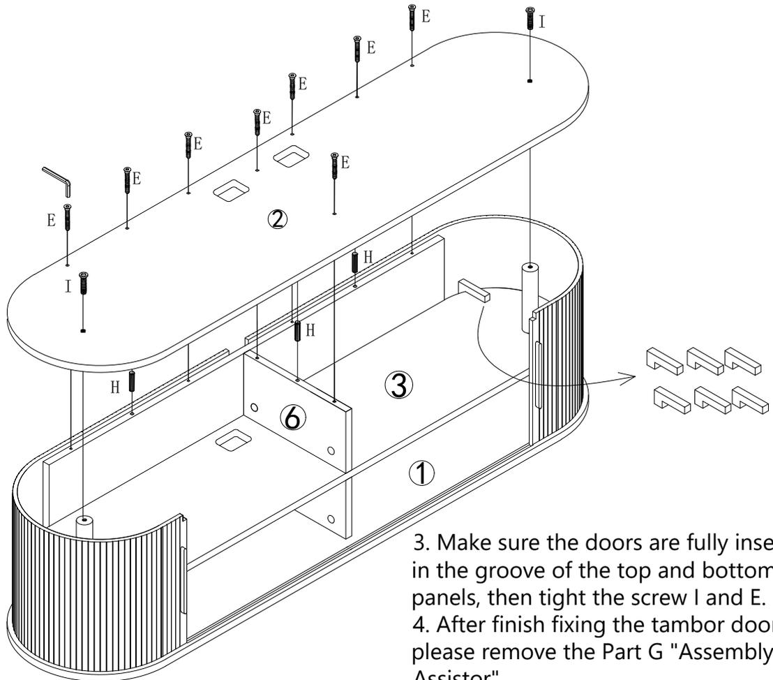
3. Make sure the doors are fully inserted in the groove of the top and bottom panels, then tight the screw I and E.
