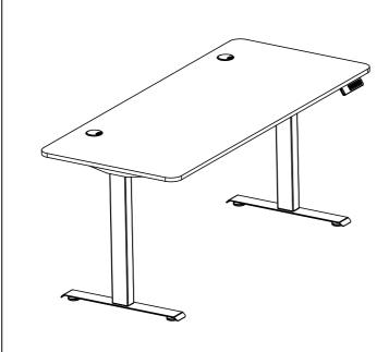
为了方便您组装,组装时请勿将螺丝锁 紧, 待全部零件锁上后, 再行锁紧。 In order to facilitate your assembly, do not assemble Tighten the screws, and when all the parts are locked, Lock it again.
