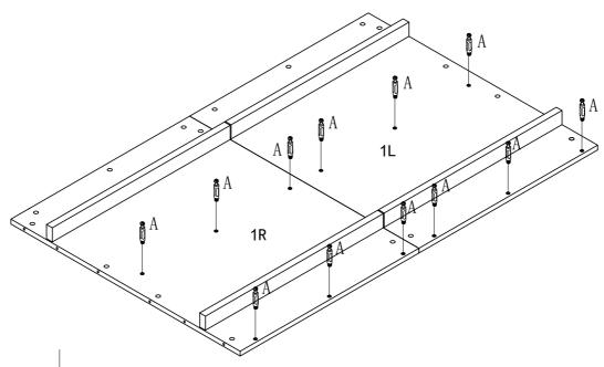
No. A Quantity:12Pcs Cam Lock Dowel 8\*28 mm
