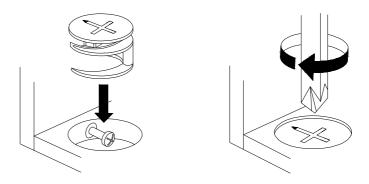
Turn cam lock clockwise to tighten.
