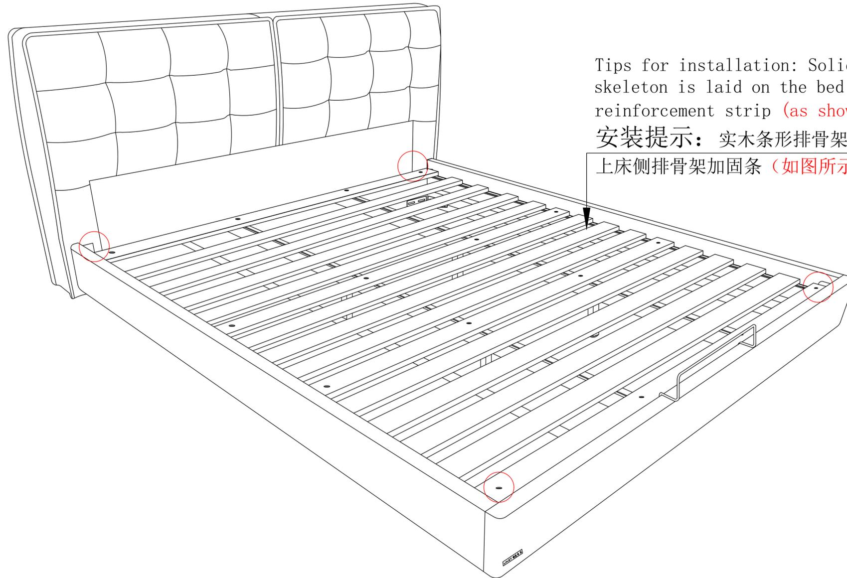
Tips for installation: Solid wood strip skeleton is laid on the bed side skeleton reinforcement strip (as shown in the figure)
