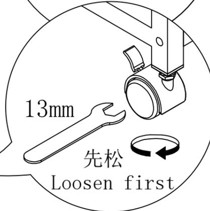
地板不平的情况而引起轮子不着地的话, 可通过用13mm扳手拧松轮子, 调整到适合高度, 然后通过用12mm扳手来向上锁紧定位螺母即可。If the wheel does not touch the ground due to the uneven floor, loosen the wheel with a 13mm wrench and adjust it to a suitable height, and then lock the locating nut with a 12mm wrench.
