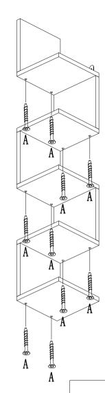
Use screws (A) with the Allen key (C) to secure each shelf in place as shown in the diagram.
