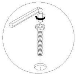
斜边内六角螺杆 Beveled hexagon socket head screw
