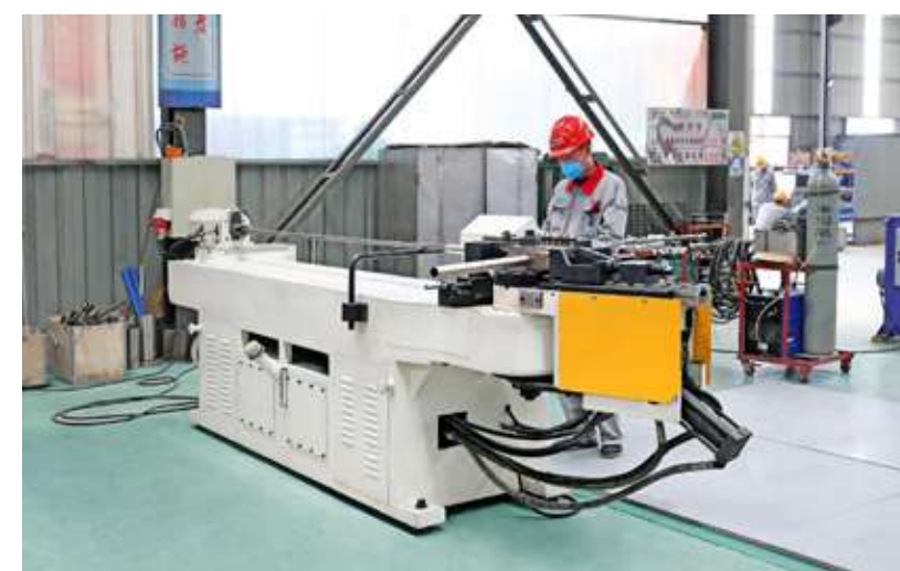
Numerical control universal pipe bender
