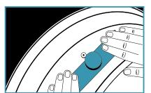
The sensor must be applied directly in the centre line of the wheel opposite the valve outlet to easily identify its position on the wheel rim when using Wheely-Safe checking tools.
