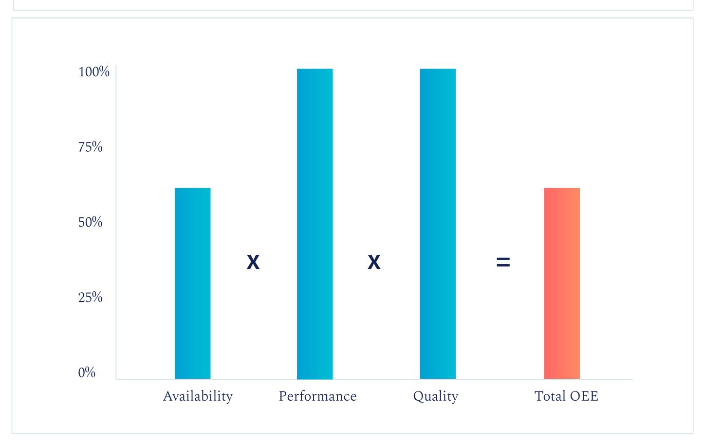
**The impact of a weak link:** Even if a factory is able to attain, for example, 100% performance and quality, if availability lags at 60% due to frequent breakdowns or operator changeover, overall OEE can never exceed 60%—the weakest of the 3 variable values.
