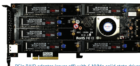
PCIe RAID adapter (cover off) with 6 NVMe solid state drives
