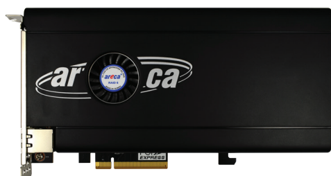
PCIe RAID adapter (cover on)
