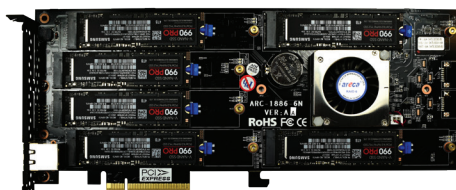
PCIe RAID adapter (cover off) with 6 NVMe solid state drives
