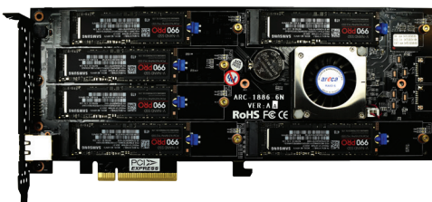
PCIe RAID adapter (cover off) showing 6 NVMe solid state drives
