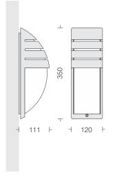
Qm23 CFW0540 123 For LED Bulb 12W/max/B22d Housing &<br/>Cover PlateCast Al in TextureDiffuserBlackMoulded Opal PC.
