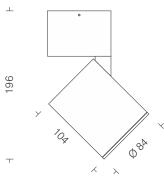
Trola 2 LDC0012 14 Power 14W LED Housing Reflector Filter Cooling COB 3000K 4000K 5000K Cast Al in White Black Faceted Mirror Bright Finish Clear Passive Heatsink in Al
