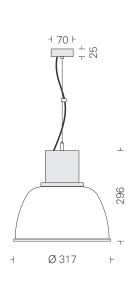
PC12 Refractor 136 CFP0001 136 For LED Bulb 17W/max/B22d Without Lens
