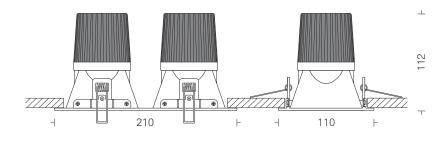
SQL Twin 1 LDR2702 215 Power 2x15W LED Dimming Housing Reflector Filter Cooling COB 03000K 04000K 05000K Tunable White Options available Cast Al in White Faceted Mirror Bright Finish Clear Passive Heatsink in Al
