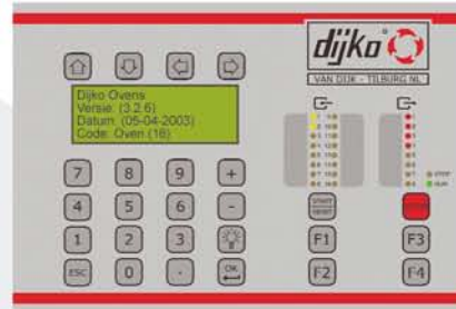
PLC - control display information screen
