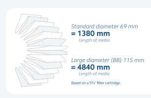
With almost 7 times the surface area of a cylindrical cartridge, the pleated construction maximises the amount of filtration media, optimising service life. The pleat pack integrity is maintained with thermally welded seams and vinyl plastisol end-caps, introducing no additives, binders or glues.
