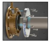
The DryMax<sup>™</sup> primary sealing components can be renewed easily with the vessel at sea. With seawater restricted by the inflatable seal the split DuraChrome<sup>™</sup> Mating Ring can be removed and the old seal ring replaced with the spare
