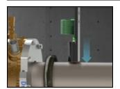
The Duramax<sup>®</sup> DryMax<sup>™</sup> Shaft Seal System includes an earthing assembly to help prevent shaft corrosion. The assembly contains a replaceable carbon brush that is spring loaded and grounded to the ship's hull.
