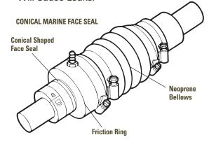
Conical marine face seals have a seal ring with a beveled face and a mating friction ring with a counter bevel. Any vibration or misalignment will cause the conical face to wear into an oval or elliptical shape. This prevents the seal from seating correctly, causing it to leak.
