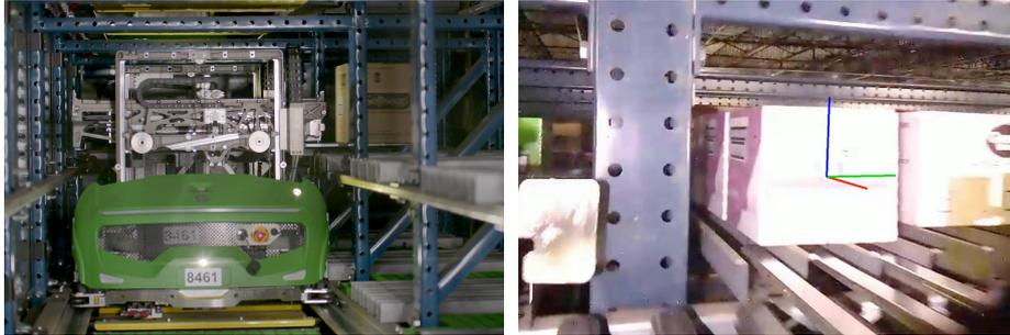
Fig. 1: (left) Robot in a Symbotic warehouse picking up a box from a shelf. (right) A real-world pick-up task using a model trained entirely in simulation and adapted with our self-supervised pipeline on unlabeled data.
