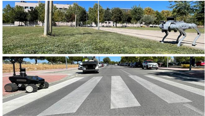
Fig. 1: Robots and scenarios used for the experimental validation of this work: Quadruped robot Go2 in a pavement-grass scenario (upper image) and wheeled robot Summit XL in a pedestrian crossing (bottom image).
