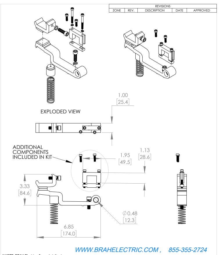
\* NOTE: BRAH Electric, aftermarket direct replacement contact kits for Westinghouse, A 200 Series, B206, 1 pole kit, suitable for use with A200, A201, A210, A211 mignetic contactors & motor starters, NEMA size 6, rated for 540A, 600V maximum
