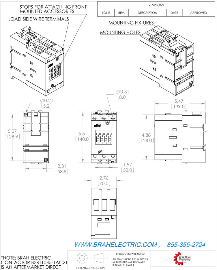
CONTACTOR B3RT1045-1AC2 IS AN AFTERMARKET DIRECT REPLACMENT FOR 3RT1045-1AC21,3RT SERIES. SUITABLE FOR USE WITH 3RT SERIES MOTOR CONTROL SYSTEMS
