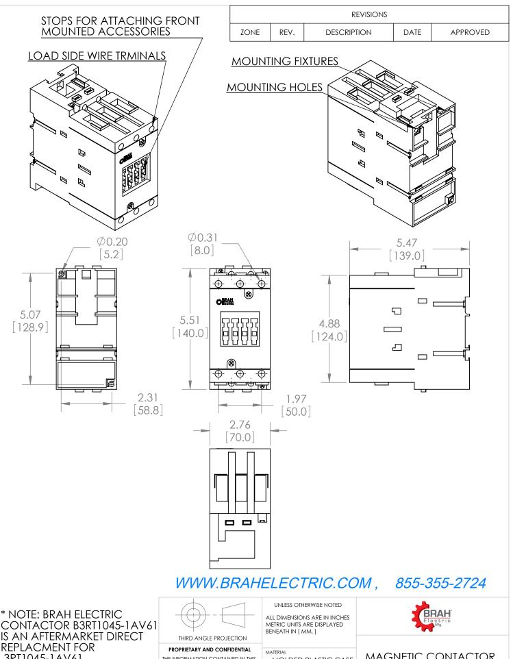
3RT1045-1AV61, 3RT SERIES. SUITABLE FOR USE WITH 3RT SERIES MOTOR CONTROL SYSTEMS
