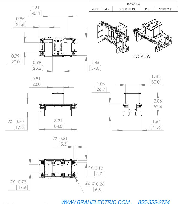
\* NOTE: BRAH ELECTRIC **COILS ARE A DIRECT** REPLACEMENT FOR SIEMENS 3RT1924-5AN21, SIRIUS, TYPE B3RT, 220V AC 50/60HZ, SUITABLE FOR USE WITH 3RT1023, 3RT1024, 3RT1025, 3RT1026 CONTACTORS
