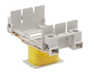
**PART NUMBER - B3RT1924-5AN21:** BRAH Electric, aftermarket direct replacement coils for Siemens 3RT1924-5AN21, Sirius, type B3RT, 220V AC 50/60Hz, suitable for use with 3RT1023, 3RT1024, 3RT1025, 3RT1026 contactors.
