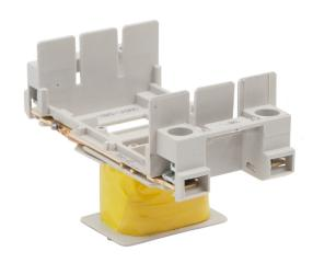
**PART NUMBER - B3RT1924-5AP61:** BRAH Electric, aftermarket direct replacement coils for Siemens 3RT1924-5AP61, Sirius, type B3RT, 220V AC 50Hz/240V AC 60Hz, suitable for use with 3RT1023, 3RT1024, 3RT1025, 3RT1026 contactors.
