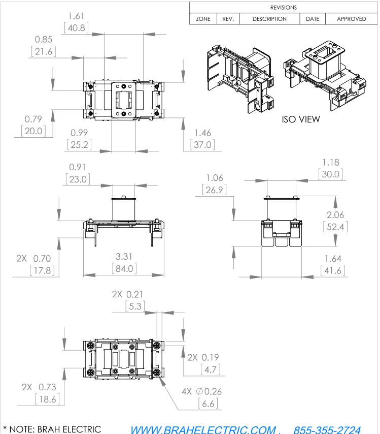
COILS ARE A DIRECT REPLACEMENT FOR SIEMENS 3RT1924-5AP61, SIRIUS, TYPE B3RT, 220V AC 50HZ / 240V AC 60HZ, SUITABLE FOR USE WITH 3RT1023, 3RT1024, 3RT1025, 3RT1026 **CONTACTORS**
