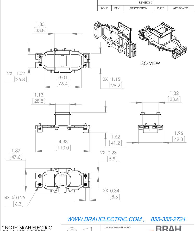
\* NOTE: BRAH ELECTRIC COILS ARE A DIRECT REPLACEMENT FOR SIEMENS 3RT1934-5AB01, SIRIUS, TYPE B3RT, 24V AC 50HZ, SUITABLE FOR USE WITH 3RT1033, 3RT1034 CONTACTORS
