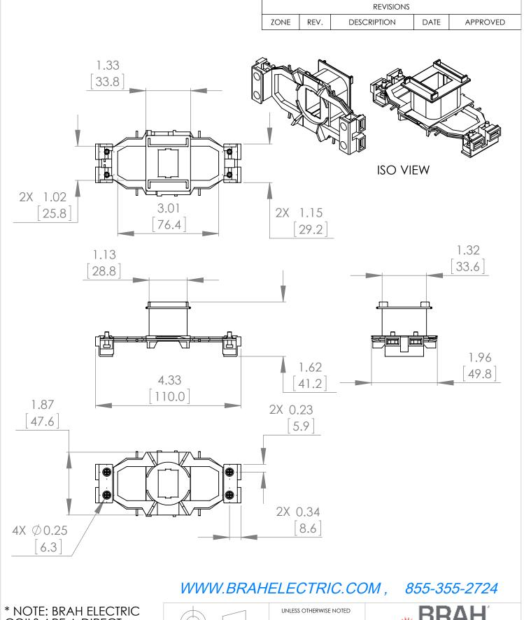
\* NOTE: BRAH ELECTRIC COILS ARE A DIRECT REPLACEMENT FOR SIEMENS 3RT1934-5AC21, SIRIUS, TYPE B3RT, 24V AC 50/60HZ, SUITABLE FOR USE WITH 3RT1033, 3RT1034 CONTACTORS
