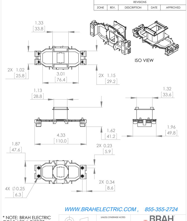
COILS ARE A DIRECT REPLACEMENT FOR SIEMENS 3RT1934-5AP61, SIRIUS, TYPE B3RT, 240V AC 50/60HZ, SUITABLE FOR USE WITH 3RT1033, 3RT1034 CONTACTORS
