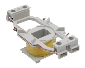
**PART NUMBER - B3RT1934-5AP61:** BRAH Electric, aftermarket direct replacement coils for Siemens 3RT1934-5AP61, Sirius, type B3RT, 240V AC 50/60Hz, suitable for use with 3RT1033, 3RT1034 contactors.
