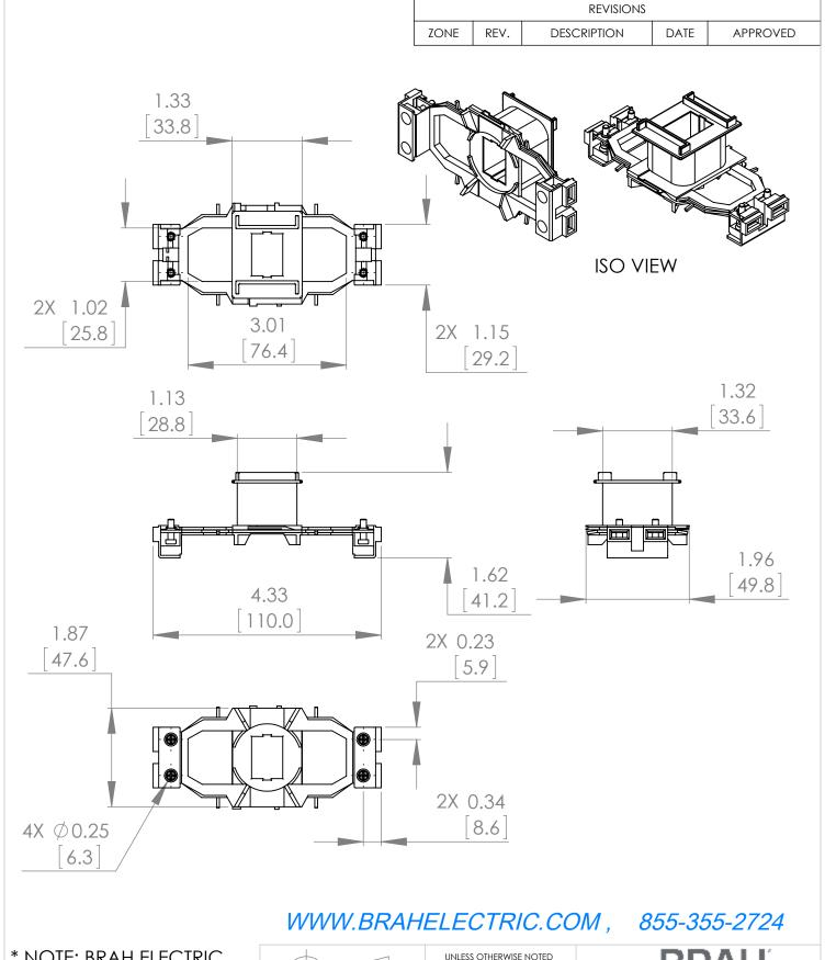
\* NOTE: BRAH ELECTRIC **COILS ARE A DIRECT** REPLACEMENT FOR SIEMENS B3RT1935-5AB01, SIRIUS, TYPE B3RT, 24V AC 50HZ, SUITABLE FOR USE WITH 3RT1035, 3RT1036 CONTACTORS
