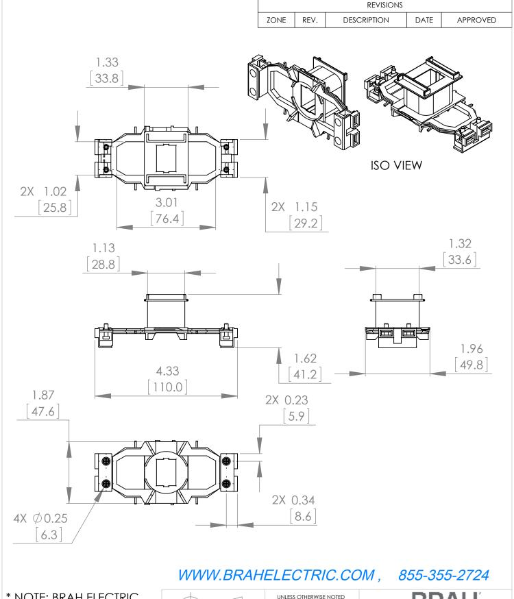
\* NOTE: BRAH ELECTRIC COILS ARE A DIRECT REPLACEMENT FOR SIEMENS B3RT1935-5AC21, SIRIUS, TYPE B3RT, 24V AC 50/60HZ, SUITABLE FOR USE WITH 3RT1035, 3RT1036 CONTACTORS
