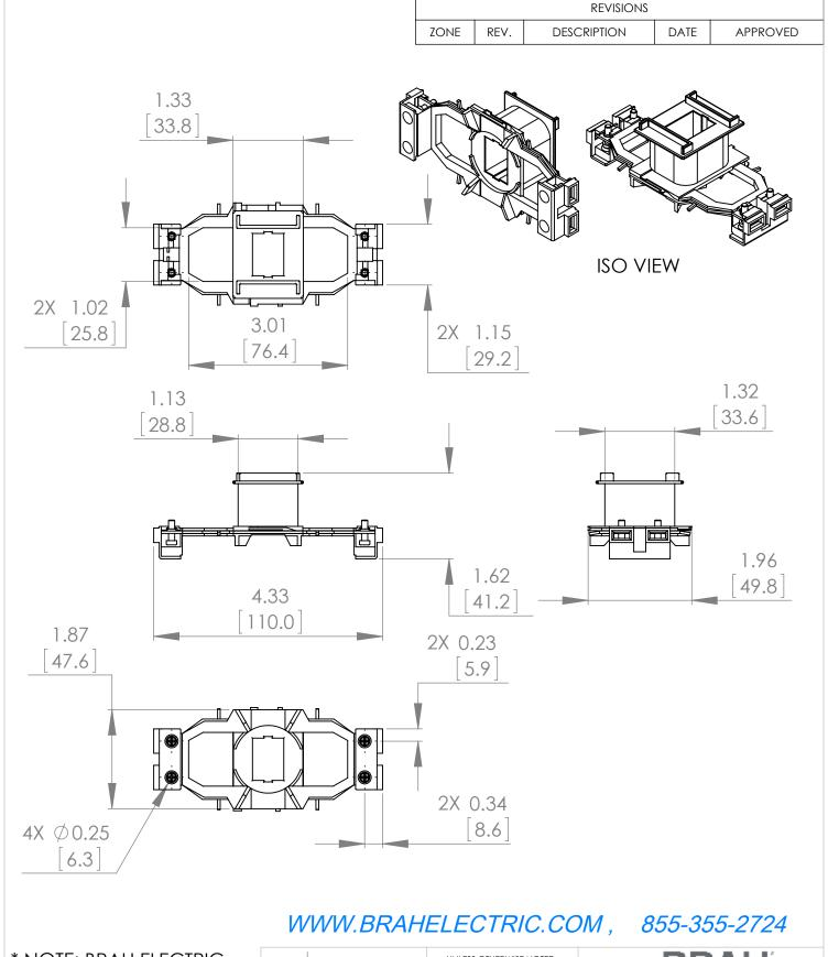
\* NOTE: BRAH ELECTRIC COILS ARE A DIRECT REPLACEMENT FOR SIEMENS B3RT1935-5AU61, SIRIUS, TYPE B3RT, 277V AC 60HZ, SUITABLE FOR USE WITH 3RT1035, 3RT1036 CONTACTORS
