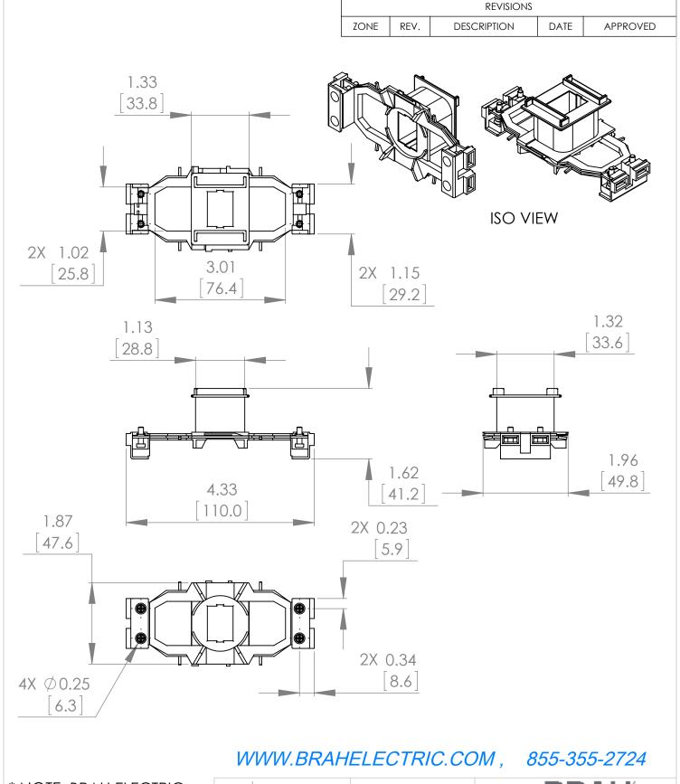
\* NOTE: BRAH ELECTRIC COILS ARE A DIRECT REPLACEMENT FOR SIEMENS B3RT1935-5AV61, SIRIUS, TYPE B3RT, 480V AC 60HZ, SUITABLE FOR USE WITH 3RT1035, 3RT1036 CONTACTORS
