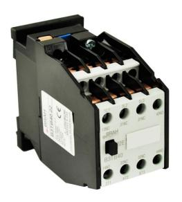
PART NUMBER-B3T41: BRAH Electric, aftermarket direct replacement contactors for Siemens 3TB41, World Series, type 3TB, 3P, 3PH, 12A, 600V, 3HP @ 230V, 7.5HP @ 460V, 10HP @ 575V, complete with 110/120V AC coil, 2 N/O - 2 N/C auxiliary contact, AC magnetic contactor, suitable for use with 3TB series motor control systems
