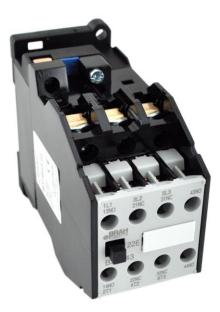
**PART NUMBER–B3T4322**: BRAH Electric, aftermarket direct replacement contactors for Siemens 3TB4322, World Series, type 3TB, 3P, 3PH, 22A, 600V, 7.5HP @ 230V, 15HP @ 460V, 20HP @ 575V, complete with 110/120V AC coil, 2 N/O - 2 N/C auxiliary contact, AC magnetic contactor, suitable for use with 3TB series motor control systems
