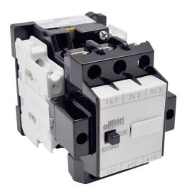
**PART NUMBER–B3TB44**: BRAH Electric, aftermarket direct replacement contactors for Siemens 3TB44, World Series, type 3TB, 3P, 3PH, 32A, 600V, 10HP @ 230V, 25HP @ 460V, 30HP @ 575V, complete with 110/120V AC coil, 2 N/O - 2 N/C auxiliary contact, AC magnetic contactor, suitable for use with 3TB series motor control systems
