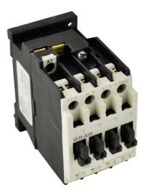
PART NUMBER – B3TF3010-0AK6: BRAH Electric, aftermarket direct replacement contactors for Siemens 3TF3010-0AK6, World Series type 3TF, 3P, 3PH, 9A, 600V, 3HP @ 230V,5HP @ 460V, 7.5HP @ 575V, complete with 110/120V AC Coil, 1 N/O auxiliary contact, AC magnetic contactor, suitable for use with 3TF series motor control systems
