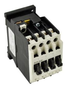
PART NUMBER – B3TF3010-0AVO: BRAH Electric, aftermarket direct replacement contactors for Siemens 3TF3010-0AVO, World Series type 3TF, 3P, 3PH, 9A, 600V, 3HP @ 230V,5HP @ 460V, 7.5HP @ 575V, complete with 480V AC Coil, 1 N/O auxiliary contact, AC magnetic contactor, suitable for use with 3TF series motor control systems
