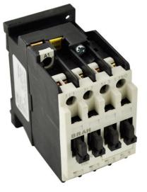
PART NUMBER – B3TF3110-0AC2: BRAH Electric, aftermarket direct replacement contactors for Siemens 3TF3110-0AC2, World Series, type 3TF, 3P, 3PH, 12A, 600V, 3HP @ 230V, 7.5HP @ 460V, 10HP @ 575V, complete with 24V AC coil, 1 N/O auxiliary contact, AC magnetic contactor, suitable for use with 3TF series motor control systems
